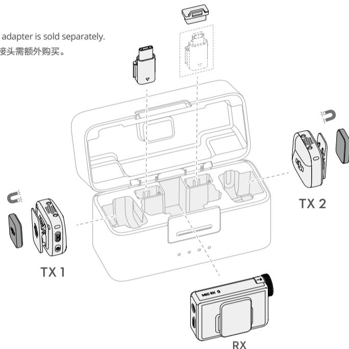
**2** Attach the TX with a clip or magnet. The windscreens reduces wind noise and can be removed when there is no wind.
